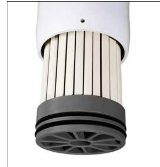
The segmented monolith contains flat sheets that are extruded and assembled to make a monolith. Nanostone Water
